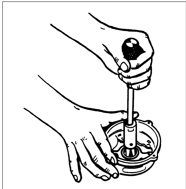
Figure 11-4. Removal of Slip Ring End Bearing
